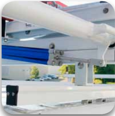
HYDRAULIC CYLINDER GREATLY REDUCES MUSCLE STRAINS
