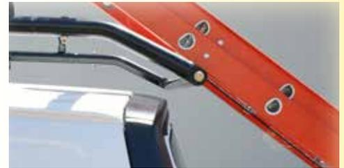
Rear roller bar makes it easier to load heavy ladders, bulky items, sheet goods and protects the top of the van.
